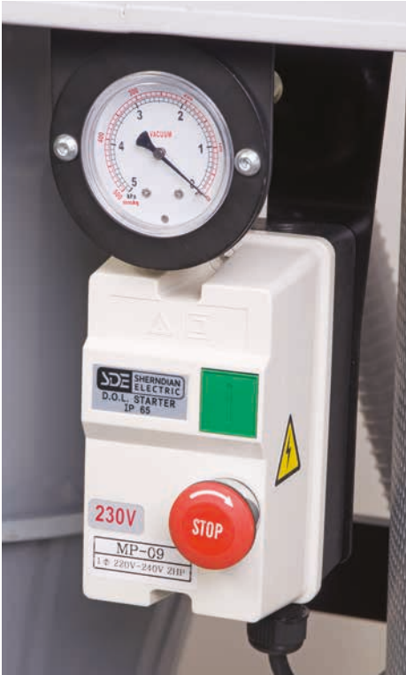
NVR Switch assembly Green (ON) Emergency Stop (Red)
